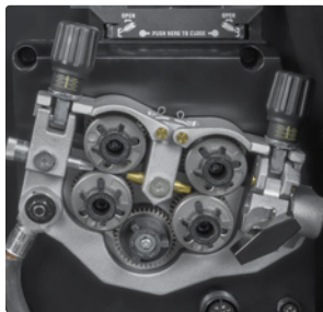
Heavy-duty aluminum four-drive-roll system.
